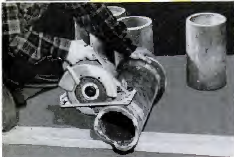
Above, note similarity of operations of cutting wood and clay tile. Saw is held in same manner. Woodcutting blade is replaced by abrasive disk for cutting tile. Right and below, saw squares up broken pieces of hollow tile and concrete for re-use
